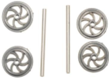
Assemble the wheels onto the axles with a flange to flange spacing of 28mm, ensuring that the flanges are inwards.
